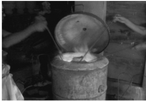
Fig. 3.3 : Photograph of the Developed Furnace during taking out of heated mould
