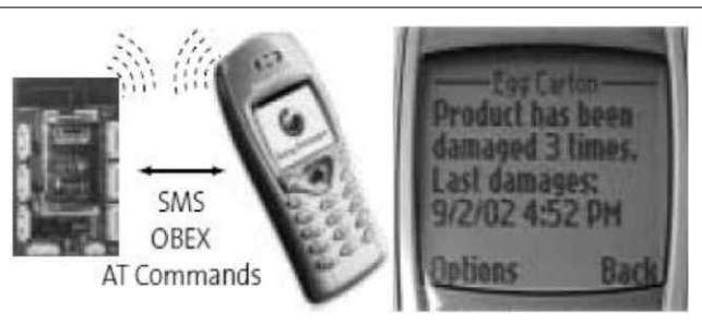
Figure 8. Product monitoring using BTnodes as smart tags and SMS via mobile phones
